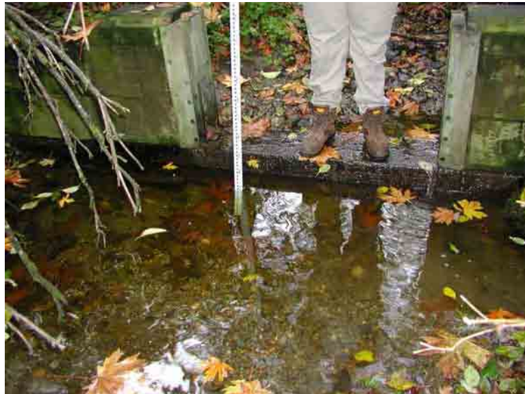
FIGURE 1.2.-- Photo taken in the winter of 2006 looking upstream at the weir pool on Mohlendorph Creek. This was the deepest spot recorded on Mohlendorph Creek. This location was dry during the summer sampling of 2005. The stream flows from the upper-center of the photo, through the weir, and into the pool at the bottom of the photo.
