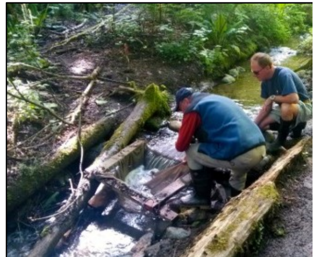
Dennis Hinton and Pete Droughon check one of the two smolt traps installed by Steev Ward to monitor out-migration. Photo courtesy Suchang Le
